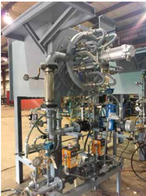
Beijing Aerospace University. Two 14MW Ultra Low NOx burner / 13ppm with FGR
