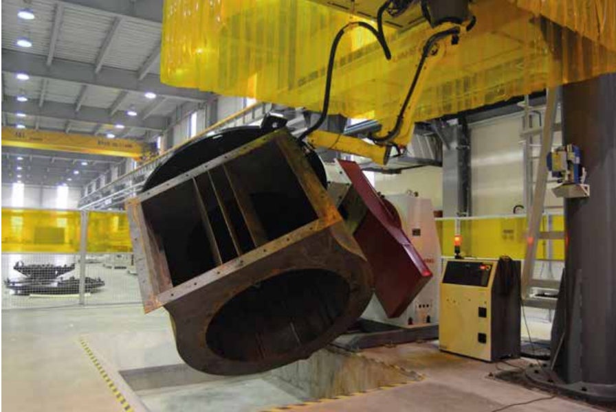
Robotic Welding at NTFB Shanghai Factory
