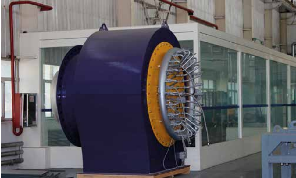
Complete Burner Assembly
